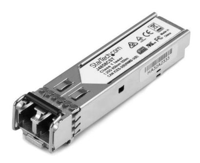
The J4858CST is an HP J4858C compatible fiber transceiver module that has been designed, programmed and tested to work with HP® brand switches and routers. It delivers dependable 1 GbE connectivity over fiber cable, for 1000BASE-SX compliant networks, with a maximum distance of up to 550 m (1804 ft).
